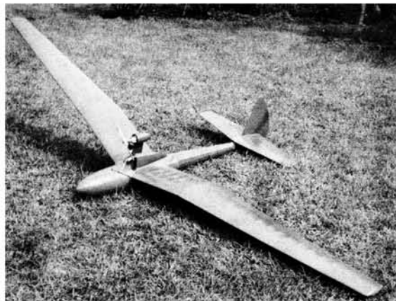
Above: High aspect ratio, sheeted wing edges, sparless. Fuselage is circular, formers on keel, 1/8" strip planked, sanded.
