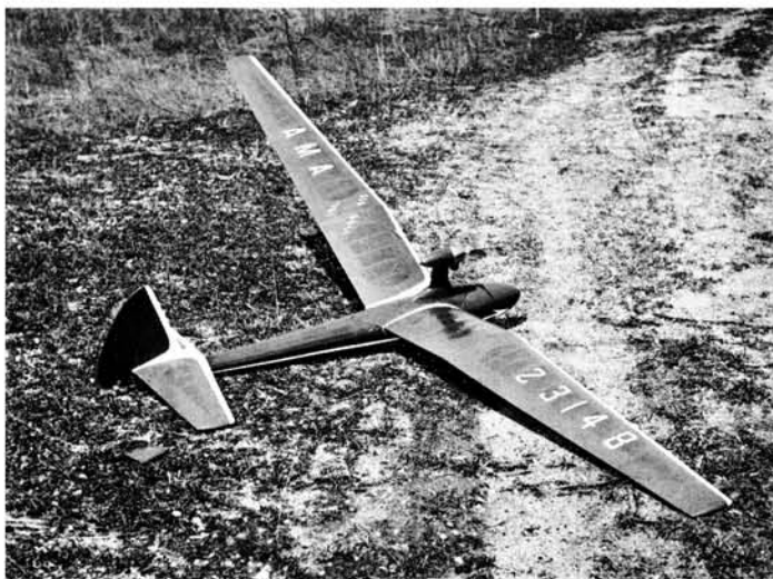
Above: A gentle gull wing lowers C.G., performed well in all flight tests. At left: Designer Bill Siegel, ex-stunt pilot, displays finished "Sea Gull".
