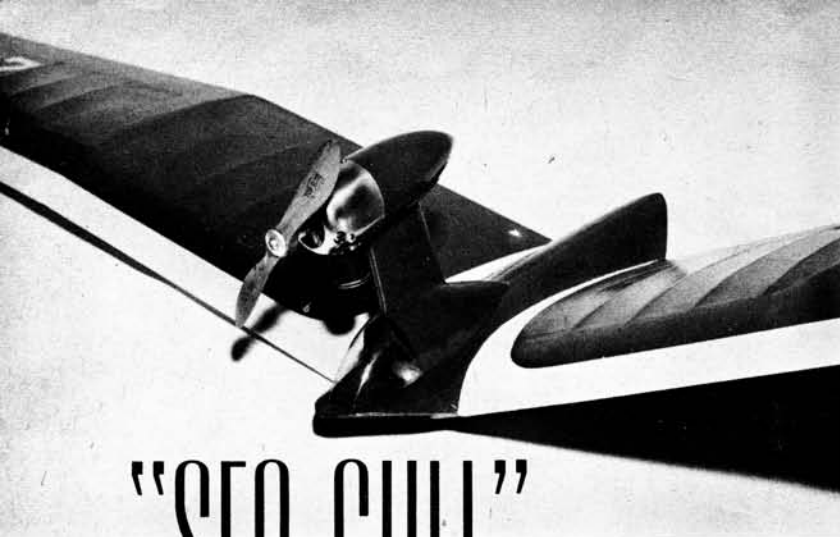
Above: High aspect ratio, sheeted wing edges, sparless. Fuselage is circular, formers on keel, 1/8" strip planked, sanded.
