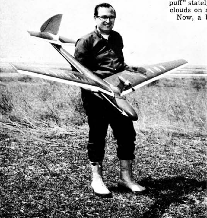
Above: A gentle gull wing lowers C.G., performed well in all flight tests. At left: Designer Bill Siegel, ex-stunt pilot, displays finished "Sea Gull".
